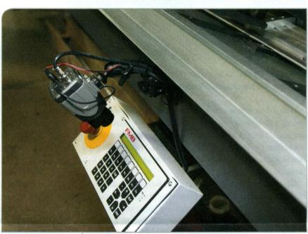
:: Monitoring the control panel on the FMB bar feeder alerts Mr. Mauro when the barstock needs to be replenished. The 42-bar magazine capacity of the feeder will generally last 4 days for a typical job.
